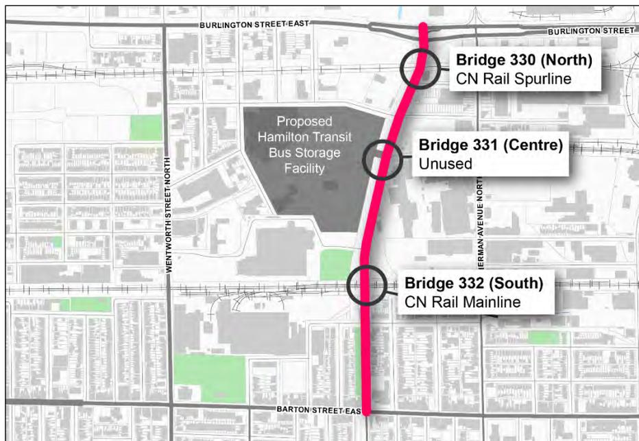
Bridge 330 has a clearance of 4.1 m, and Bridge 332 has a clearance of 4.2 ms. Both are lower than the MTO standard of 4.8 m of clearance.
