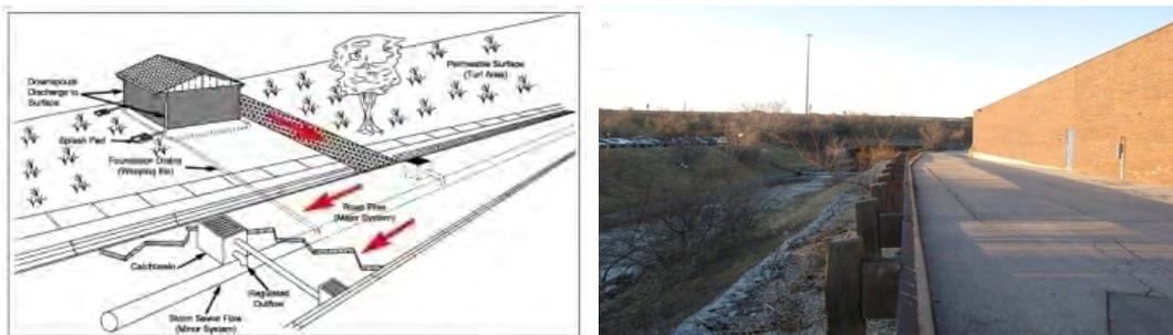
(From L to R: Conceptual Curb and Gutter, Concrete Lined Surface Channel)
