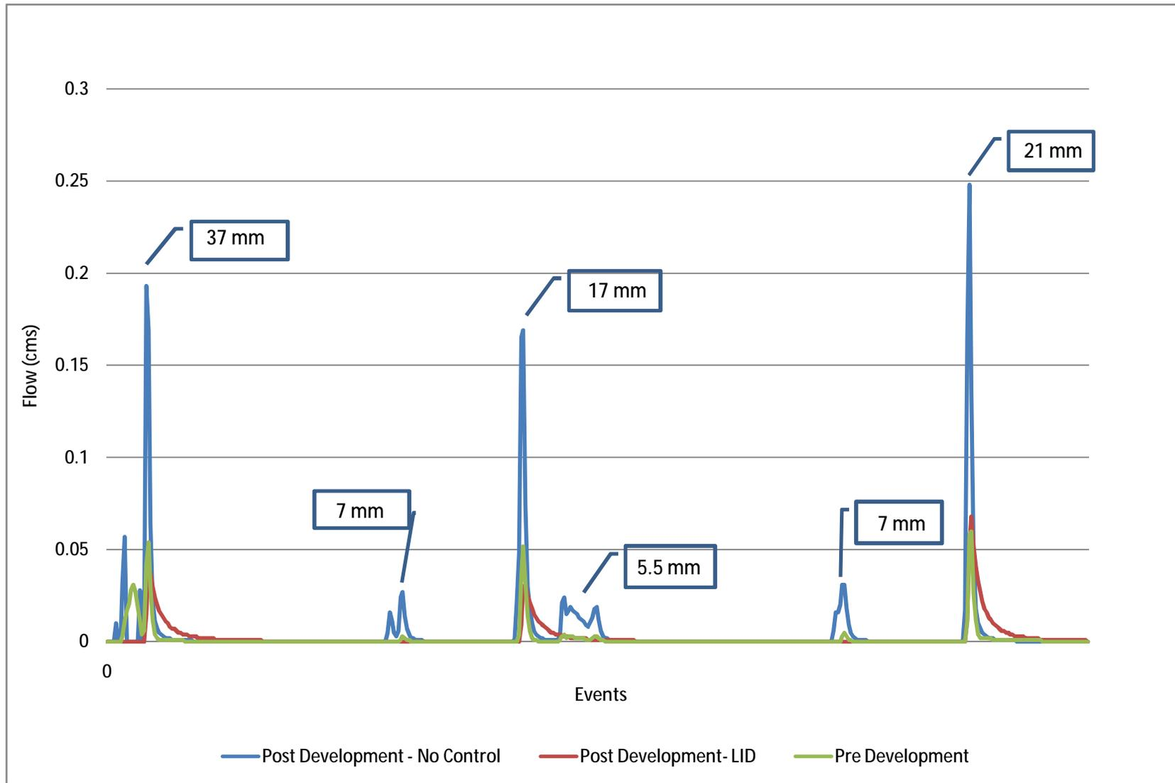
**Figure 4.20:** Site Plan Test Case – Continuous Modeling results for Various Rainfall Events (April 16 – May 4, 1992)
