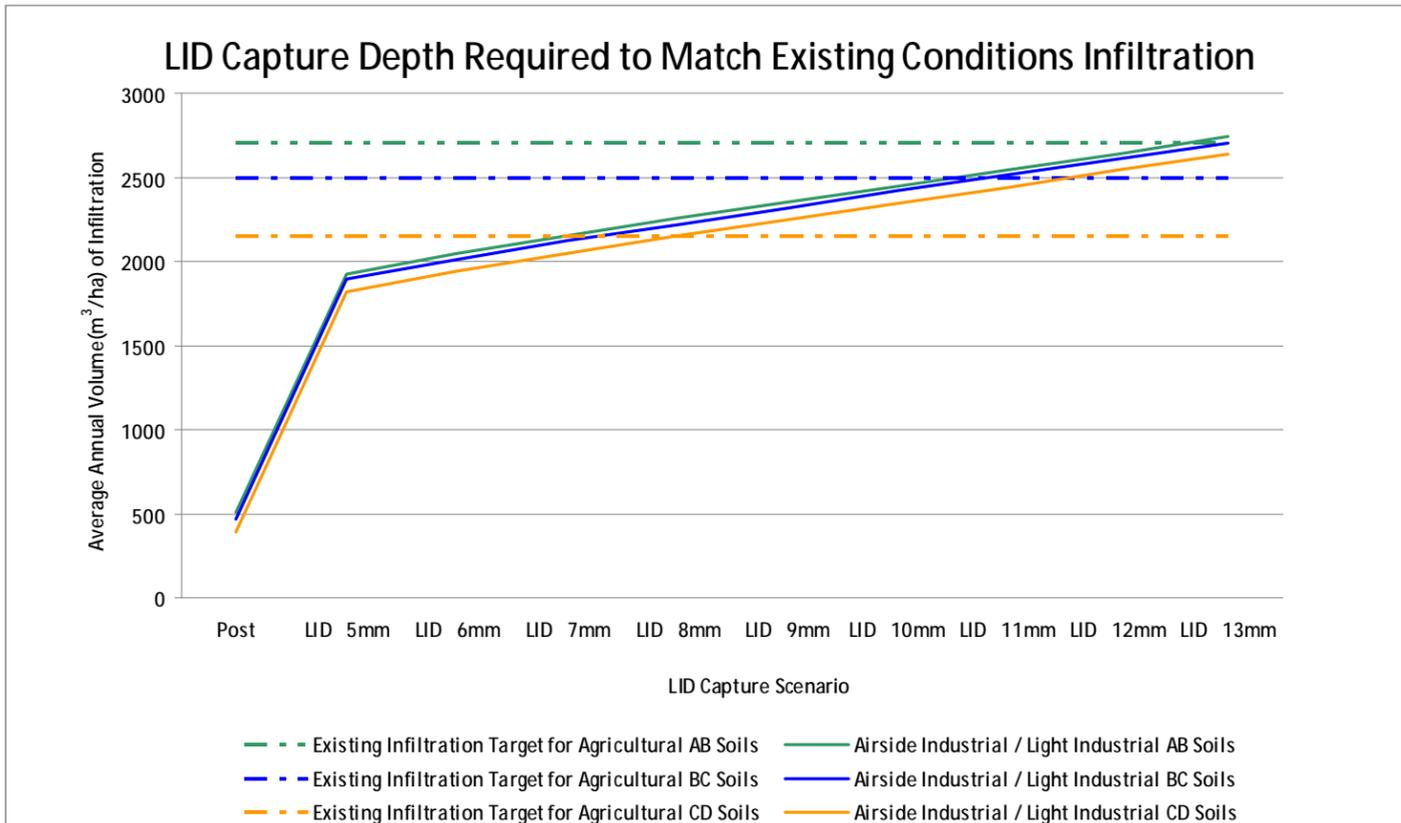
Figure 4.5: Required LID Capture Depths for Airside Industrial / Light Industrial
