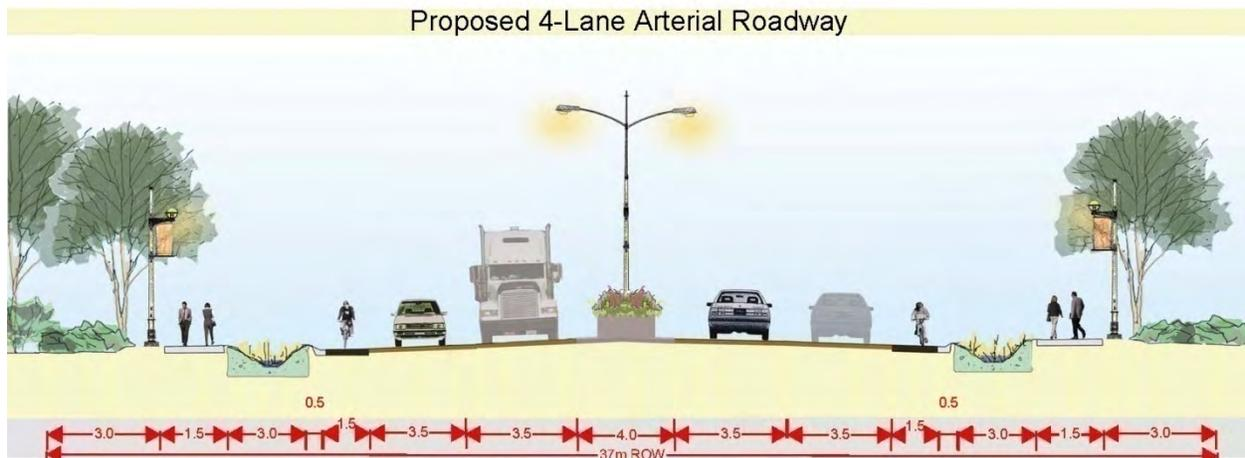
**Figure 3.1:** Proposed -4 Lane Arterial Roadway with Raised Median and 3m allowance for LID conveyance Controls
