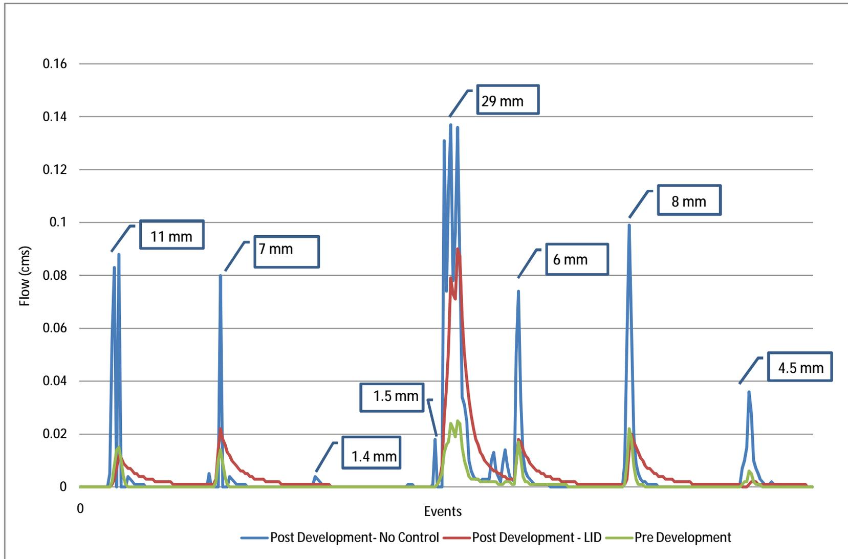
**Figure 4.19:** Site Plan Test Case – Continuous Modeling results for Various Rainfall Events (Oct 8 – Oct 21, 1992)
