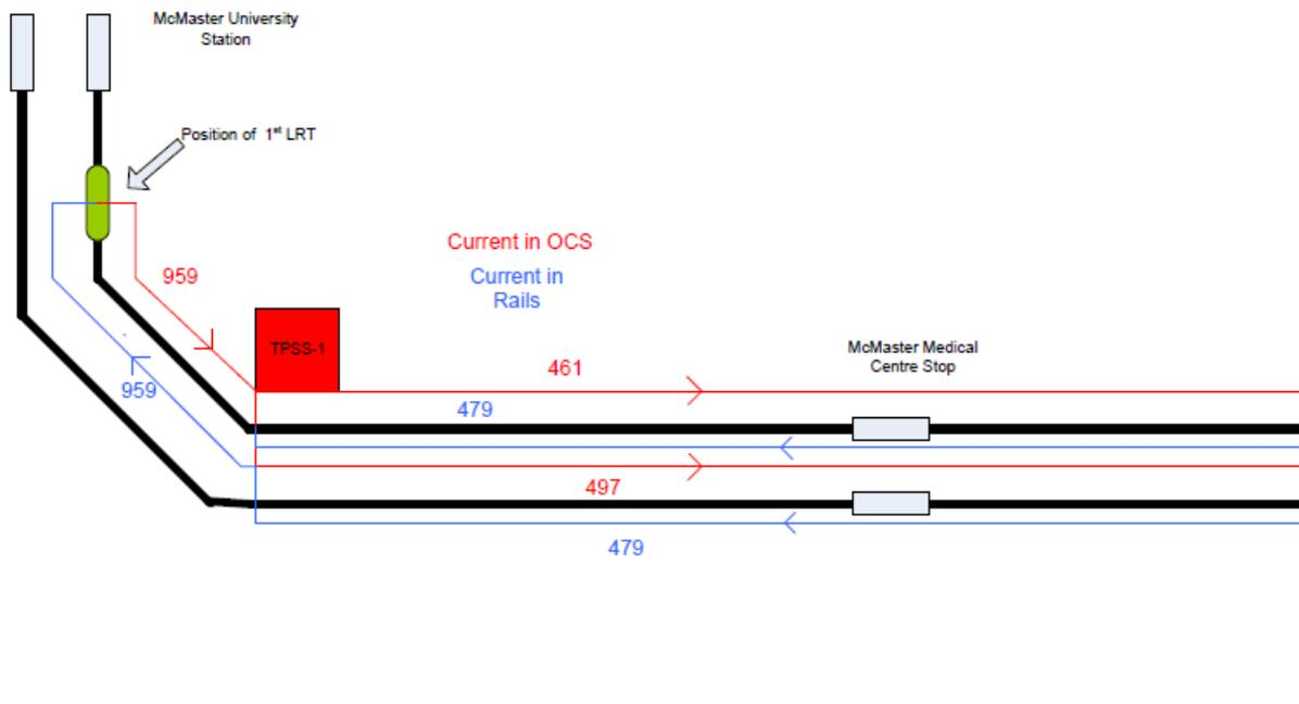
**Figure 5: Current Magnitude and Direction, Normal Operation**
