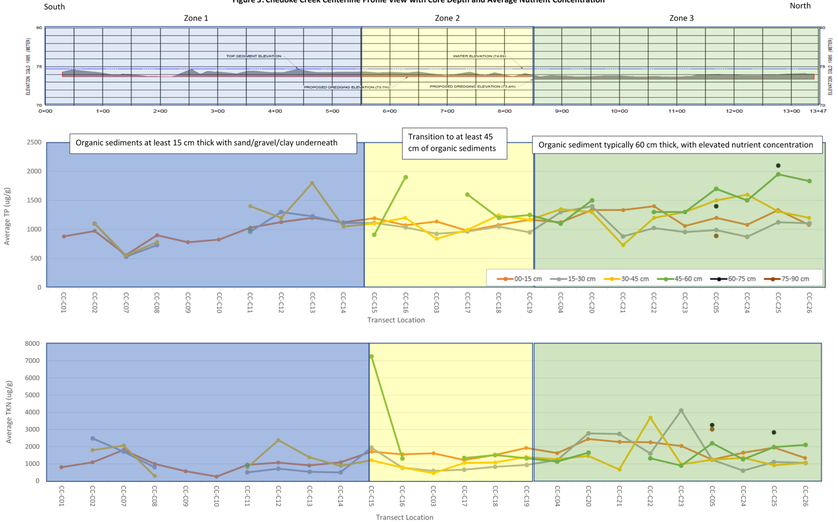
Figure 3. Chedoke Creek Centerline Profile View with Core Depth and Average Nutrient Concentration
