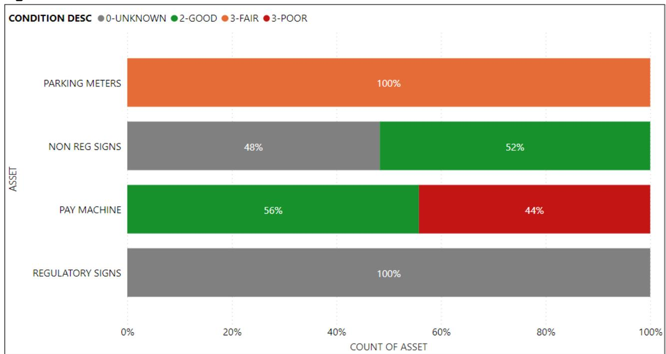
Parking meter condition has been assumed to be in Fair condition based on subject matter expert opinion. These assets are patrolled regularly as part of coin collection activities and non-functioning parking meters are generally repaired within 24 hours when reported. In addition, the internal mechanisms can be replaced separately from the external metal housing and mechanisms. The data confidence for condition is evaluated as low as it is based on assumption and subject matter expert opinion.
