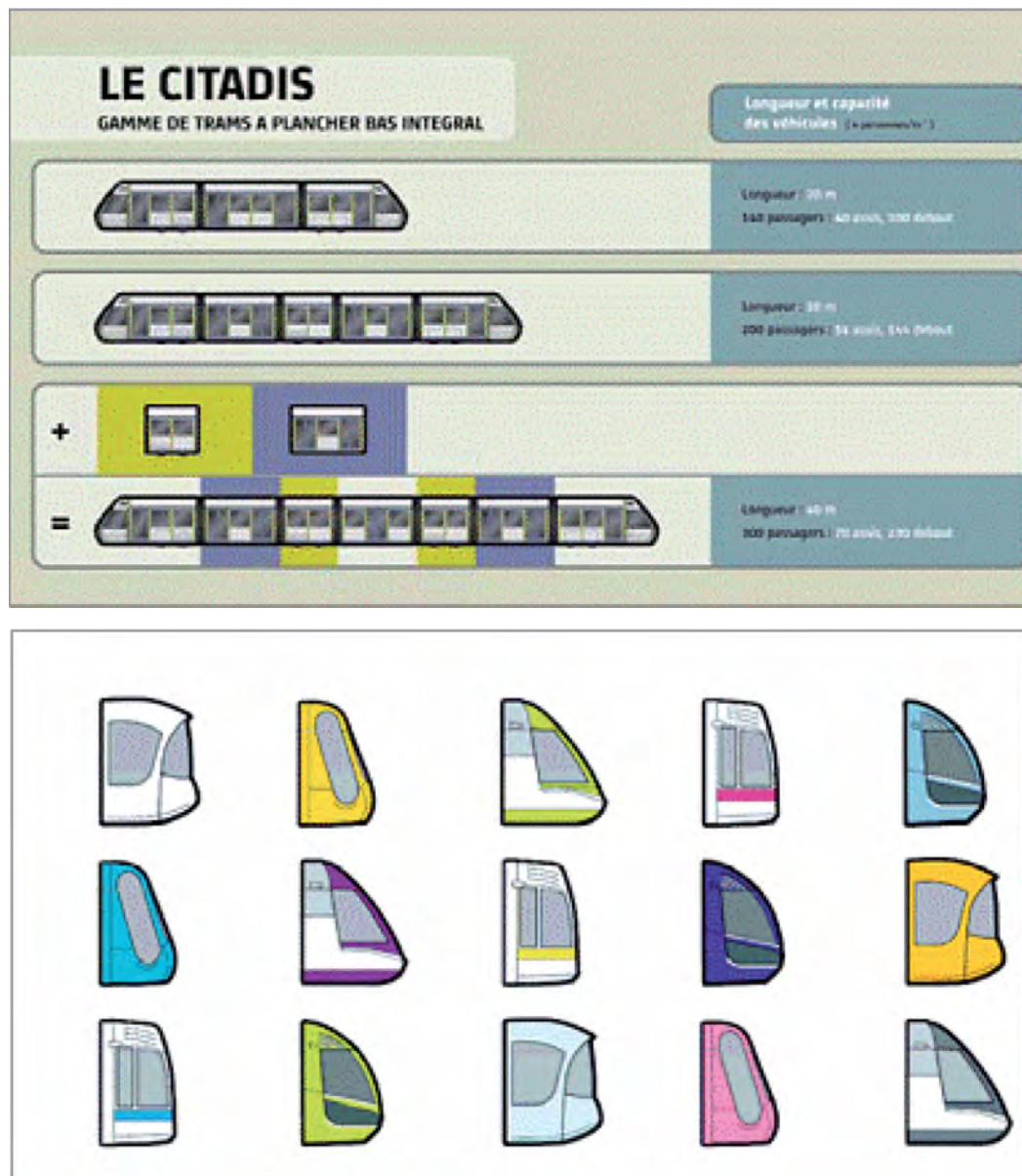
FIGURE A.14 CITADIS MODULAR VEHICLE OPTIONS AND ALTERNATIVE VEHICLE END DESIGNS
