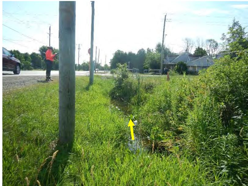
The Barton Street crossing appeared to be causing a slight backwater, as evidenced by the standing water upstream of the structure.
