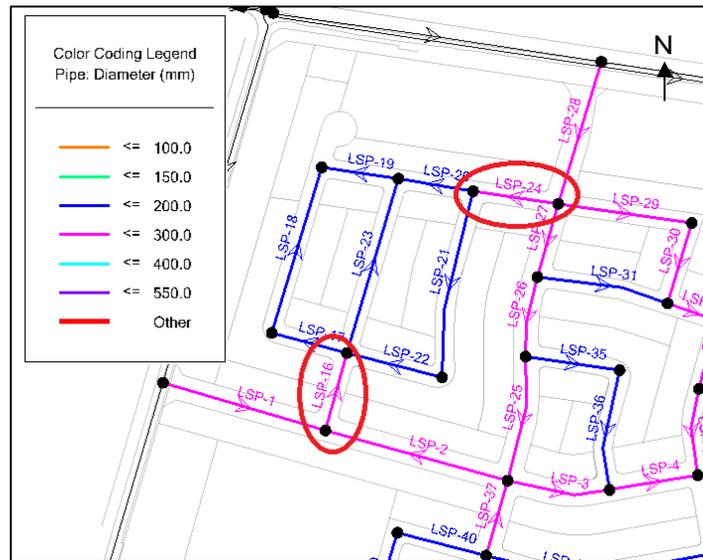
**Figure 4 – Possible Watermain Upgrades (LSP-24 and LSP-16) to Increase AFF (Circled in Red)**
