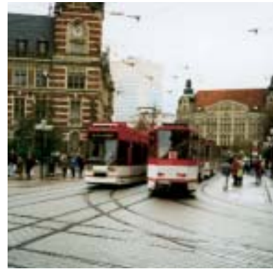
Erfurt/Germany, Anger. By continuously undersealing the Ri60 rails, vibrations were reduced by 40%.
