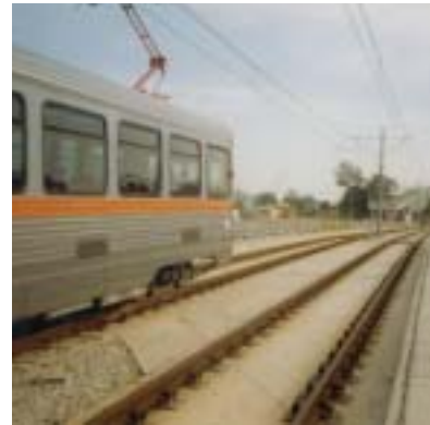
Tuen Mun LRT/Hongkong. Discrete fixation with Pandrol baseplates and Icosit® KC flexible grout.
