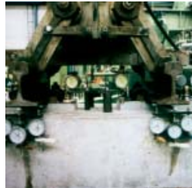
Dynamic testing on pulsating load test rig
