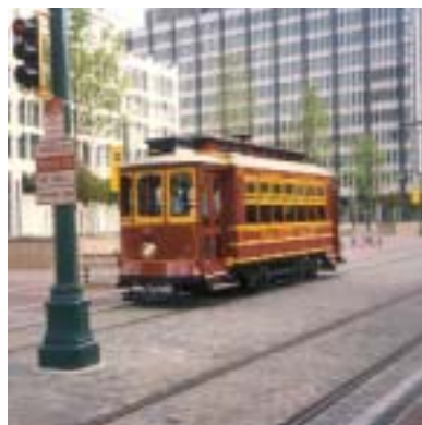
Memphis/Tennessee, USA. Embedded (floating) rail design. The very basic suspension system of heritage trams requires efficient damping. Suppression of stray currents to protect buried utility cables, pipes etc. is also a major concern.
