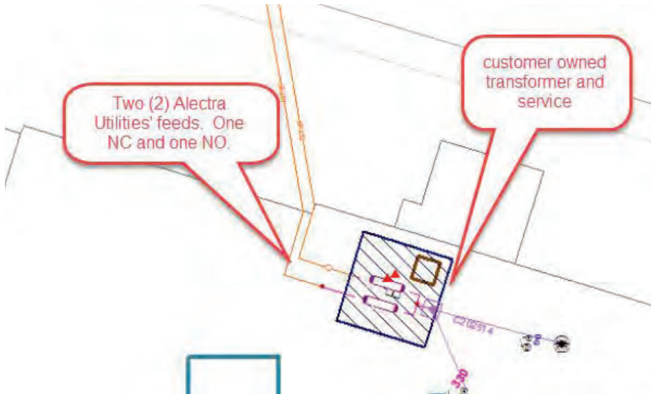
Figure 2-7 Horizon Utilities – plan showing power supply location for the 330 Wentworth Street site.
