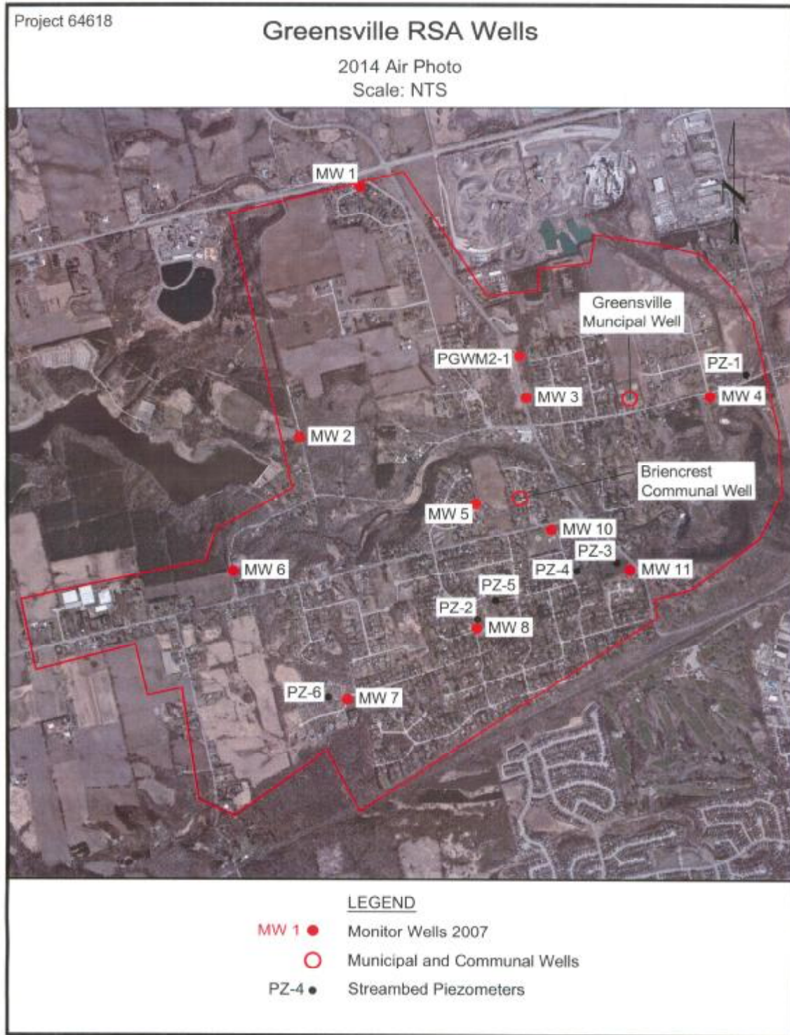
Figure 4.4.8: Locations of 2007 Monitor Wells, Greensville Municipal Well (Drilled 1972, Water Works Approval 1975), the Briencrest Communal Well (1957) and streambed piezometers
