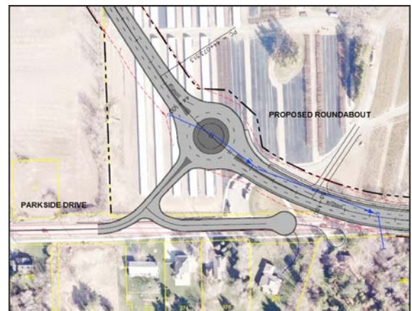
Exhibit 6-22: Parkside Drive realignment at West Roundabout
