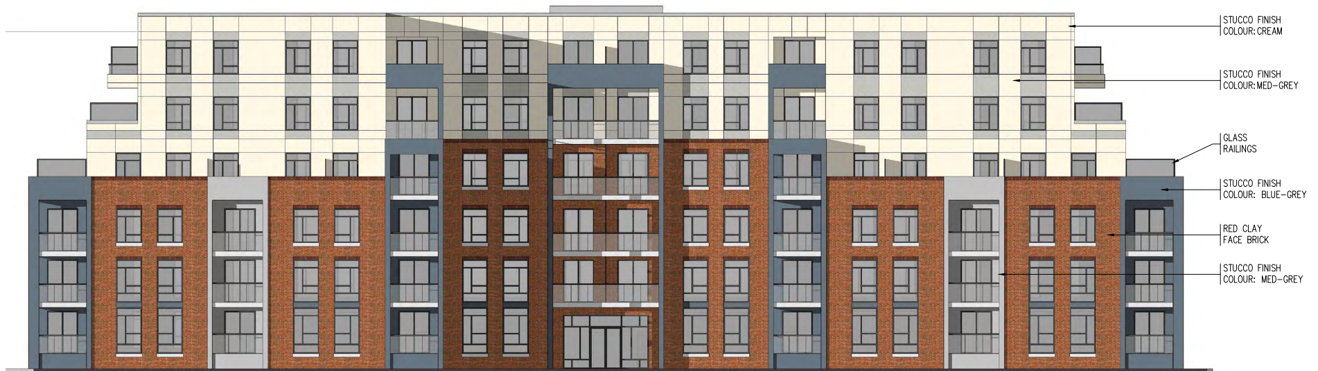
Fig.26: Front elevation showing building materials
