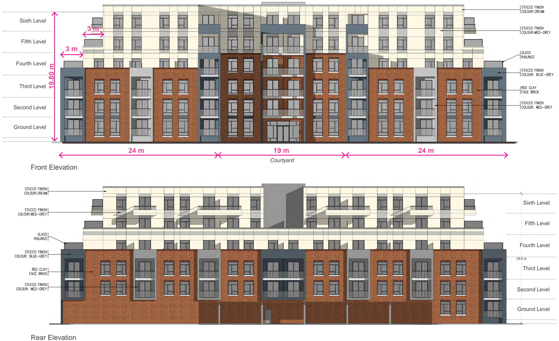
Fig.18: Elevations prepared by Lintack Architects Inc.
