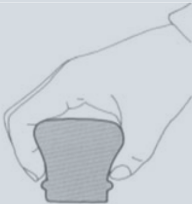
HAND RAIL INEFFECTIVE PINCH GRIP
