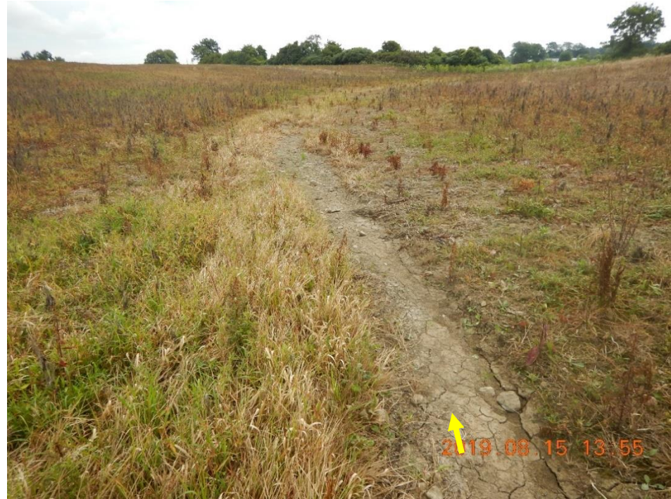
Bed and banks were mostly composed of the same material as the agricultural fields, a clay, silt, sand mixture, although some cobbles were present.
