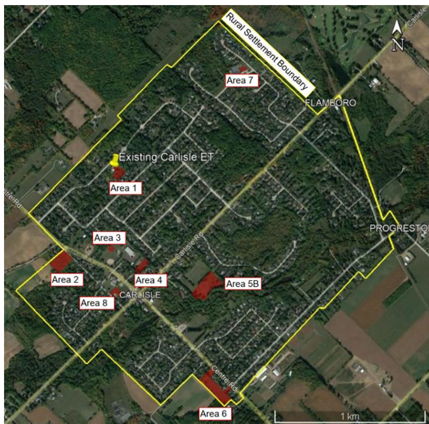
Figure 4.1 Long-List of Alternative Water Storage Site Locations
