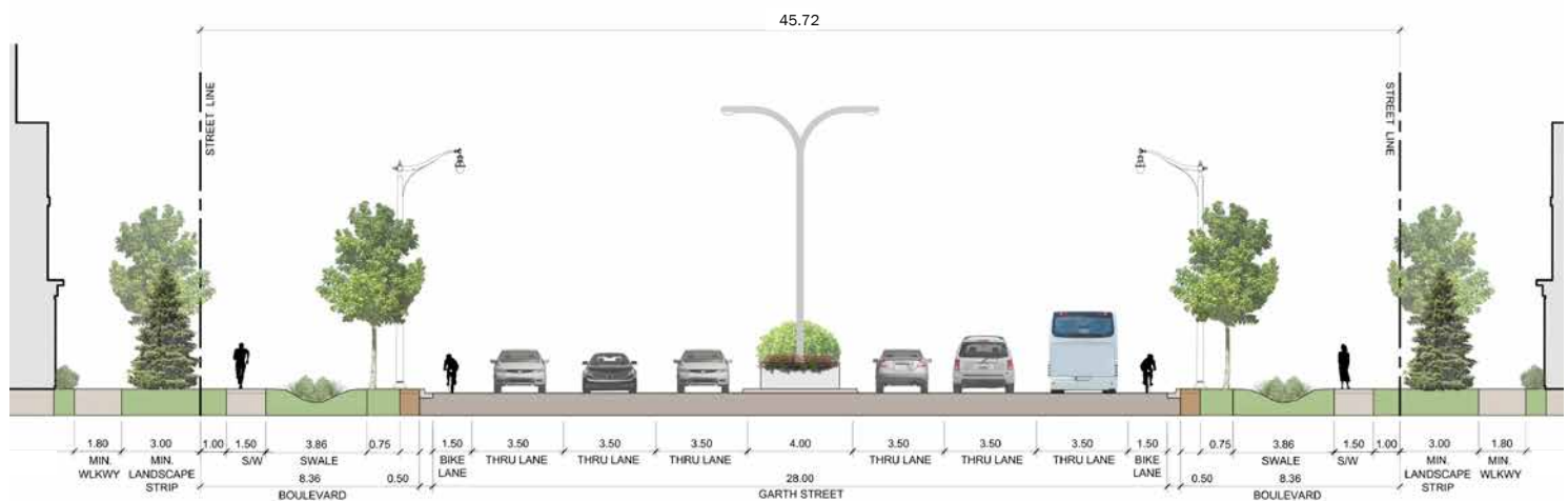
Fig. 4.1.1c - Garth Street Minor Arterial Road (Street "A") Cross Section through Employment Area.
