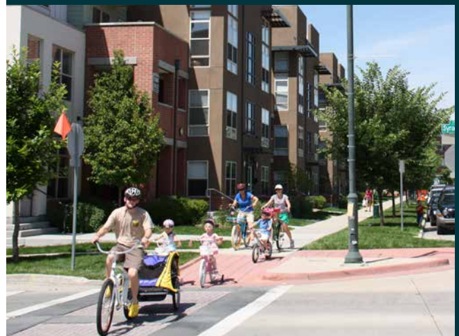
Fig. 4.1.2e - Image example of pedestrian crossing with textured paving to enhance visibility.
