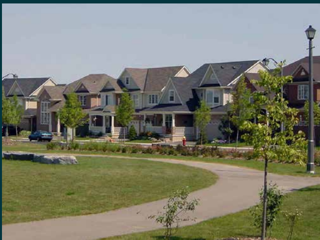
Fig. 4.3.3a - Image example showing a variety of roof forms, including the use of gables and dormers, porch projections, balconies, etc
