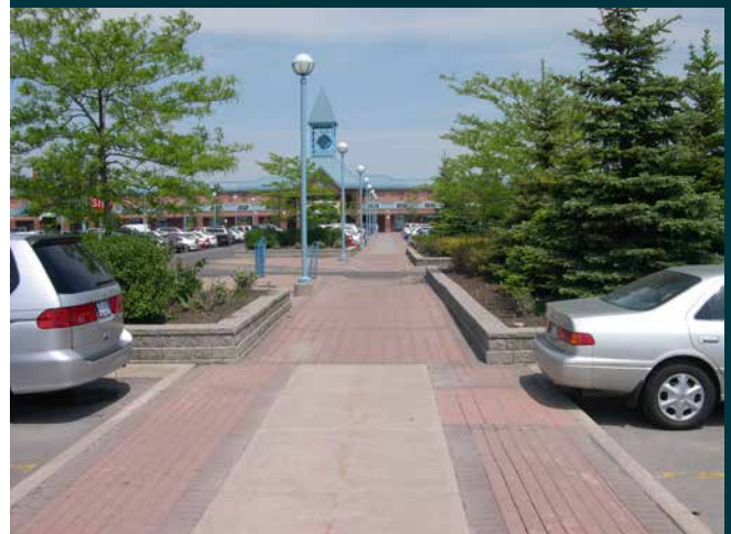
Fig. 4.5.7a - Image example of direct and safe pedestrian connection through a parking lot.
