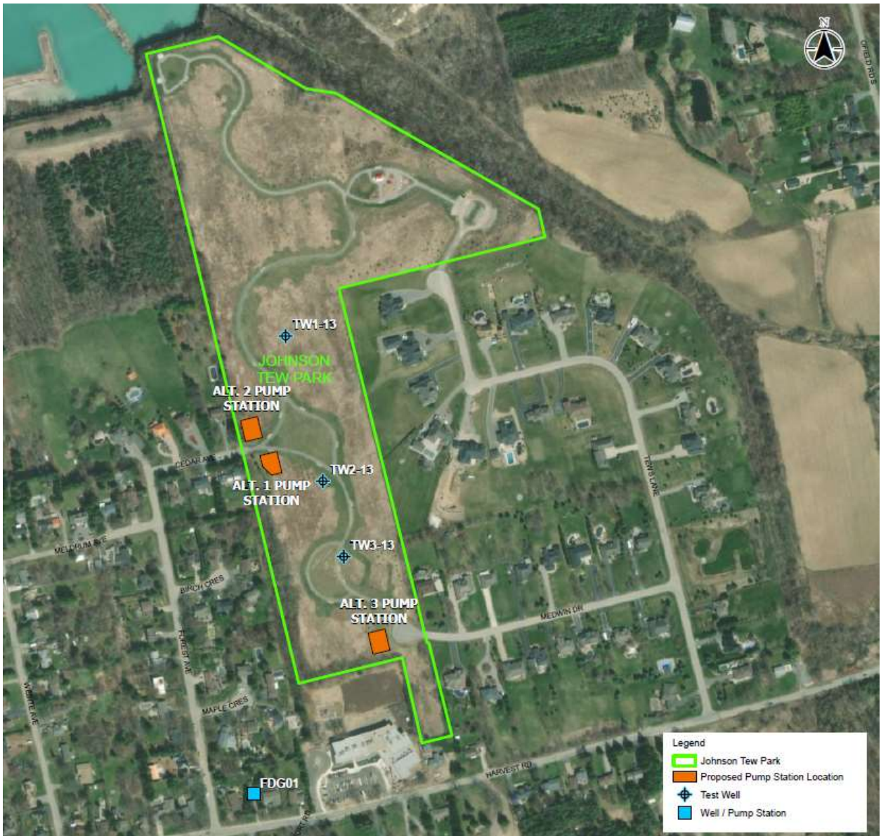
Figure 8: Well and Pump Station Alternative Locations
