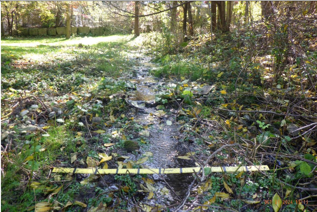
The drainage feature was observed to be flowing with a lack of defined bed or banks. As a result the bed and bank substrate was observed to consist primarily of rootlets, silt, and sand.
