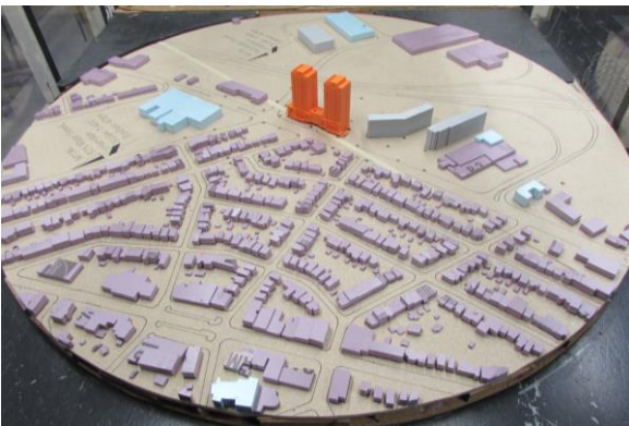
Image 3A: Wind Tunnel Model of the Site and Existing Surrounding Buildings
