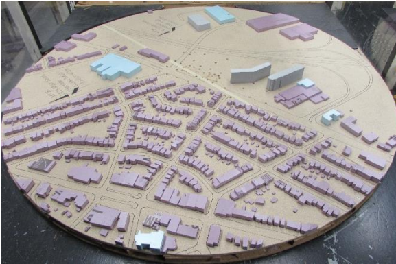
Image 3A: Wind Tunnel Model of the Site and Existing Surrounding Buildings
