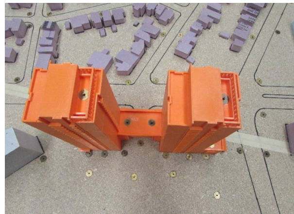
Image 3B: Wind Tunnel Model of the Proposed + Existing Surrounding Buildings
