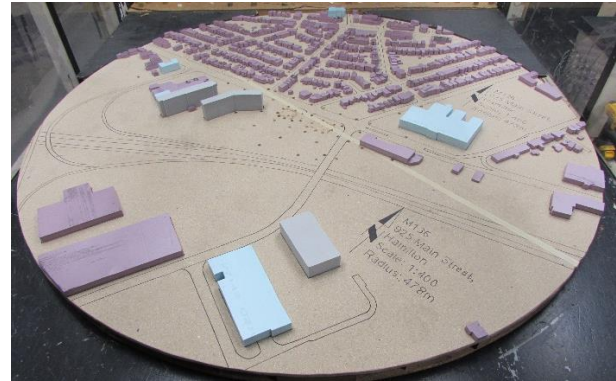
Image 3A: Wind Tunnel Model of the Site and Existing Surrounding Buildings
