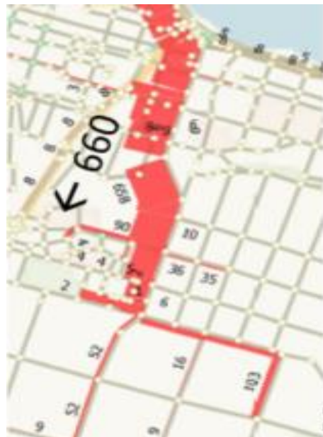
Corridor Ridership Forecasted by City of Hamilton Model on Southbound Centennial Road (ppppd)
