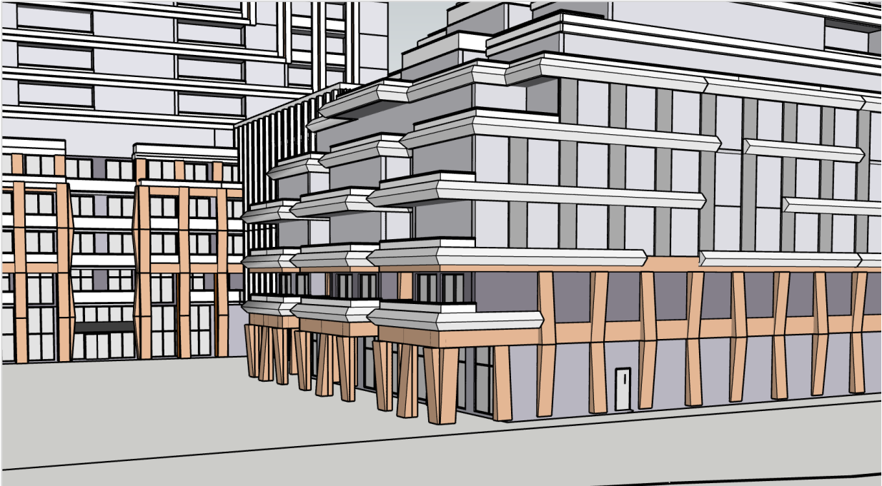
Image 5B: Overhang to the North of Tower A to Improve Conditions in the Area
